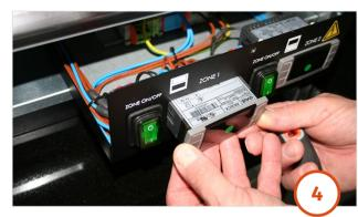
Push the new Dixell controller into the housing in the control panel.
