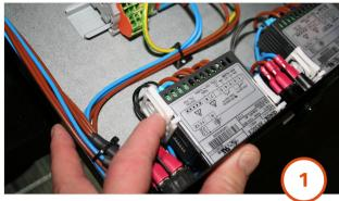
Push in the centre of both of the white clips and slide towards the rear of the unit to remove them.
