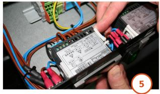
Refit the white clips by sliding them onto the back of the Dixell controller, slide them to the front to hold it firmly in position.
