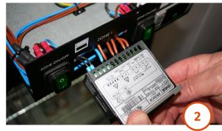
Pull the Dixell controller towards you out of the control panel.
