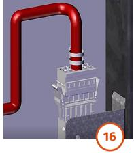
Plug the fan cable back into the wiring loom.
