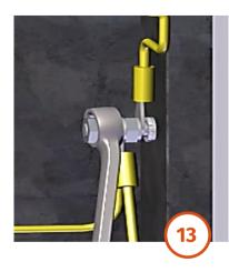
Ensure that the safety earth link is refitted before reenergising the unit.
