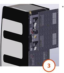
Remove top rear back panel and lower ones (as required) by pushing them up and away from the unit.
