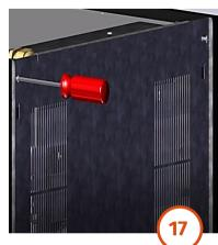
Replace all applicable back panels, ensuring that all M4 fixings are refitted to the top rear back panel.
