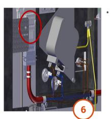
Remove the blank off plug and keep to one side for replacement fan plate.
