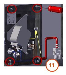
Refit the four M5 fixings into the fan plate using a 3mm hex key.
