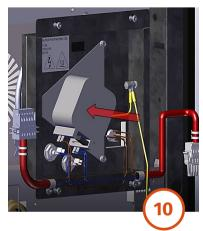
Fit the replacement fan plate into the rear back panel.
